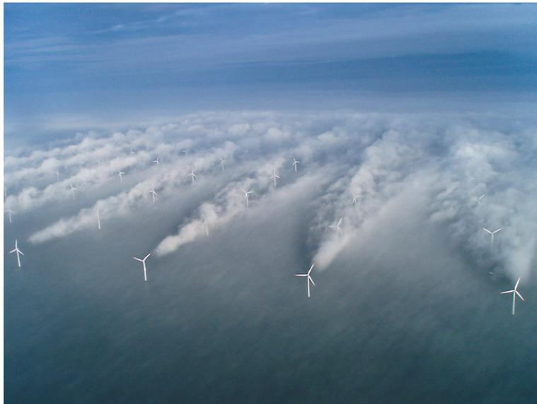
Figure 8: Rare weather condition visualizing turbulences of the turbines.
