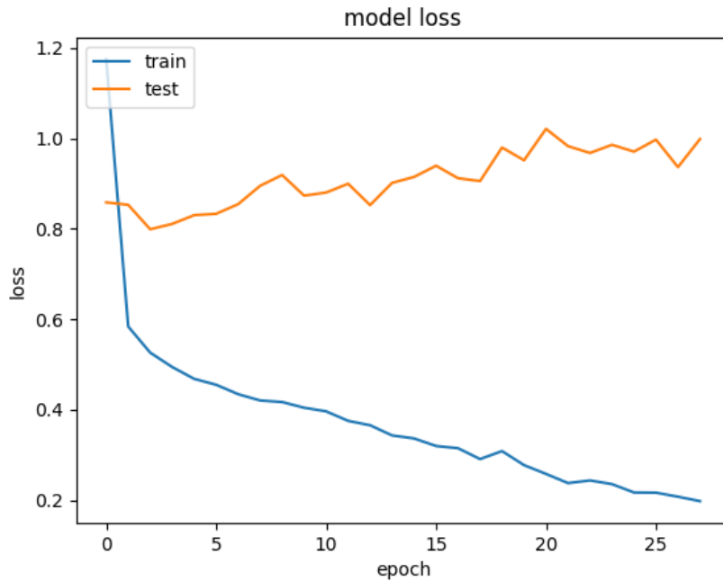
Figure 15: Training process of the 300/300/300/150 RNN model with leaky ReLU; the model shows signs of overfitting, since the training error decreases, converges and reaches fairly good results, whereas the testing error raises with every epoch
