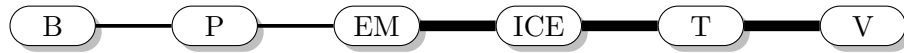
Figure 2.2: Mild parallel hybrid configuration; B - battery, P - power converter, EM - electrical motor, ICE - internal combustion engine, T - transmission, V - axles and vehicle; bold lines - mechanical link, solid lines - electrical link.
