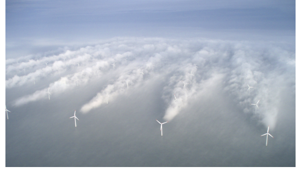
(b) Extraordinary weather conditions resulted in condensation of the very humid air, revealing the turbulence patterns behind the wind turbines [6] Picture by Christian Steiness (12.02.2008)
