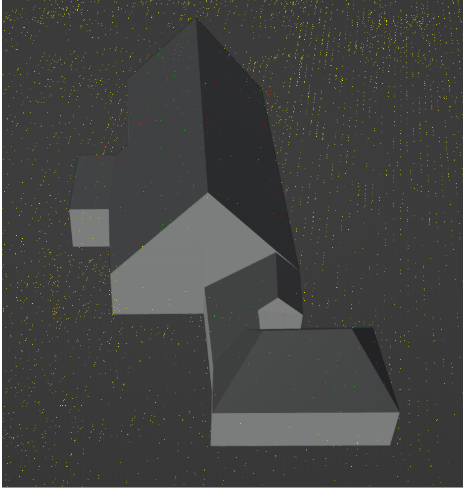
Figure 2: Point classification example: green=roof surface, red=obstacle, yellow=environment
