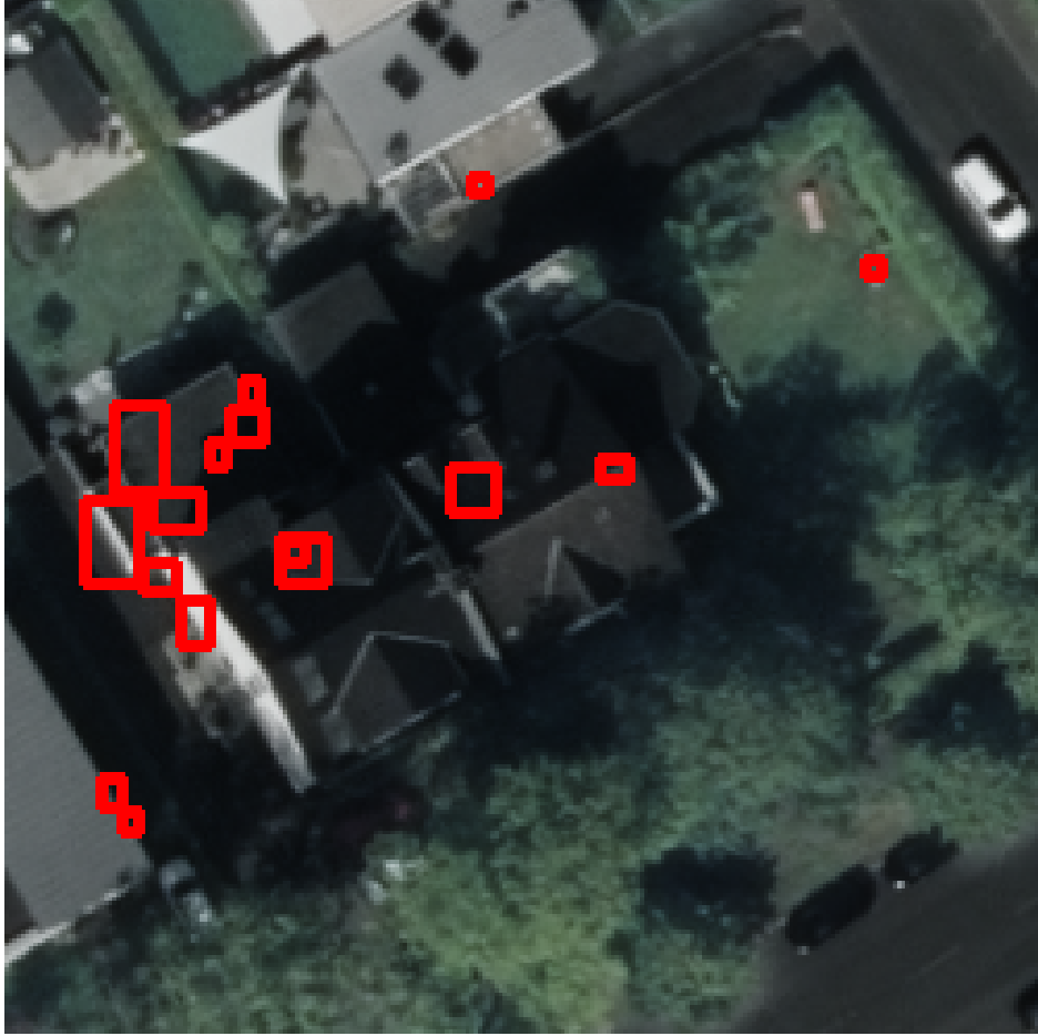
Figure 4: Image-based obstacle detection example: Aerial image with detected obstacles marked as red rectangles
