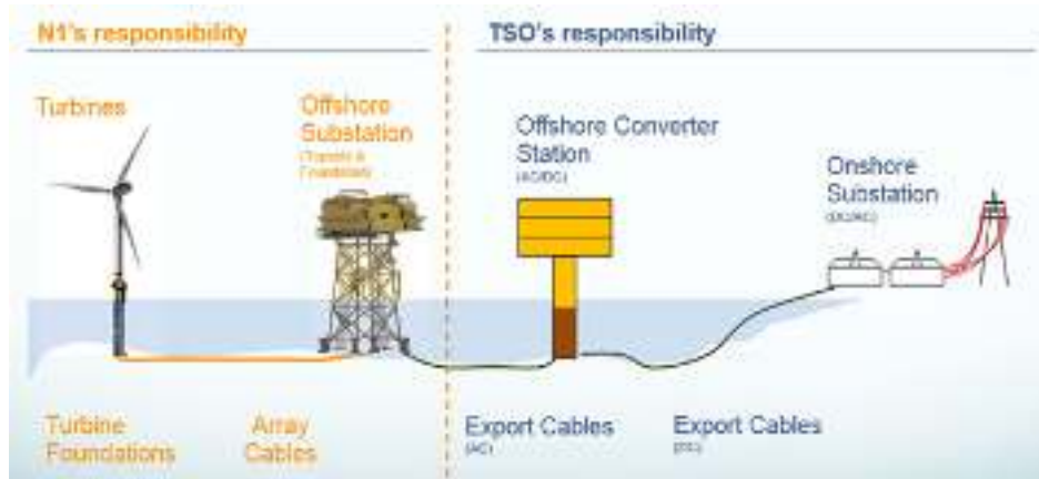
Figure 23: Overview of the different cable distributor stations on- and off-shore. The Offshore Substation is relevant for the optimization of the cable lengths in this thesis, as it connects the cable network to the individual turbines. Source: [1].
