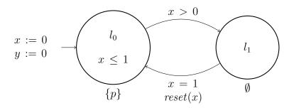
Removing syntactic sugar from  $\varphi$  yields  $\varphi = A(true \ U^{\leq 2} \ p)$  and finally removing time parameters yields  $\hat{\varphi} = A(true \ U \ ((y \leq 2) \land p))).$
