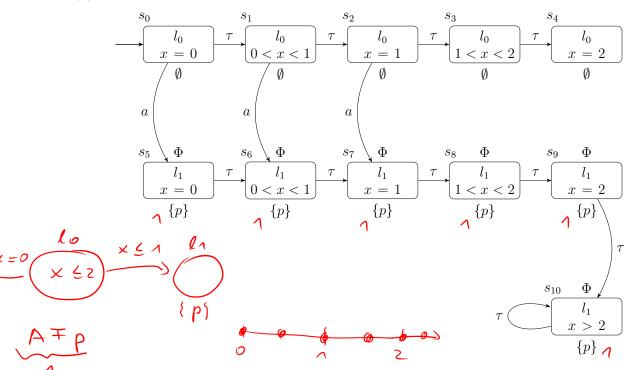
(c) Yes,  $\mathcal{T}$  has time-lock paths. Clearly,  $s_0 \to s_1 \to s_2 \to s_3 \to s_4$  is a finite path of  $RTS(\mathcal{T}, true)$ , it reflects the time-lock path  $(l_0, \nu) \xrightarrow{2} (l_0, \nu')$  with  $\nu(x) = 0$  and  $\nu'(x) = 2$ . For this Zeno-free model, we can see it on the deadlock state  $s_4$  without any outgoing transition.
