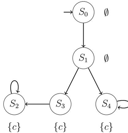
Decide whether  $TS \models \Phi$  where  $\Phi = EFAGc$ . Please sketch the main steps of the CTL model-checking algorithm.
